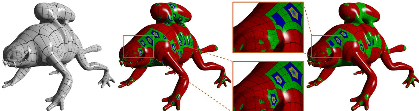
**Figure 1:** Rendering of the Frog model (left), using feature-adaptive subdivision [Nießner et al. 2012a] takes 0.68ms (middle); our method only takes 0.36ms by performing locally adaptive subdivision (right); colors denote different subdivision levels.
