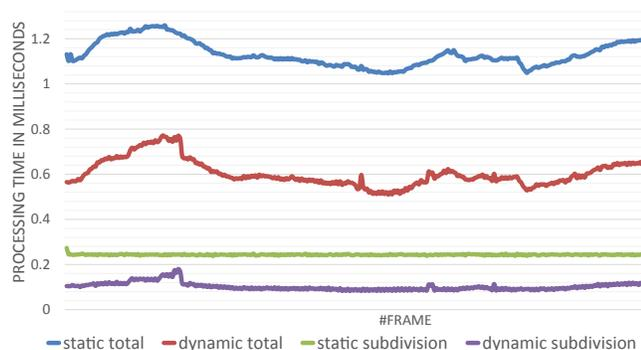
**Figure 11:** Performance comparison between static and dynamic feature-adaptive subdivision measuring the processing time during a camera flight through the terrain scene shown in Fig 10.
