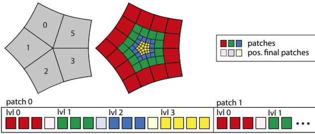
**Figure 7:** Memory layout of the patch table buffer with three subdivision levels. We store all subdivision tables and render patches around an extraordinary vertex sorted by level and order within each patch. This includes a final patch at each level for rendering when no further subdivision is necessary.
