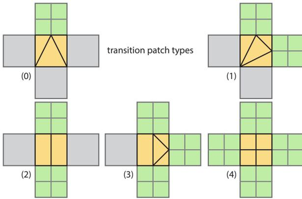
**Figure 3:** Transition patch types of feature-adaptive subdivision. These patches are used to bridge transitions between different subdivision levels where T-junctions would cause cracks otherwise. Transition patches are colored yellow, regular patches of the coarser subdivision level gray, and those of the next finer level green.
