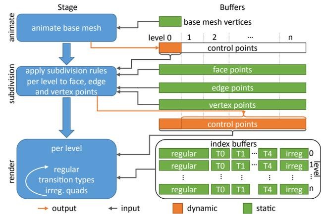
**Figure 2:** Overview of the original feature-adaptive subdivision algorithm; processing stages are shown on the left and data structures on the right.
