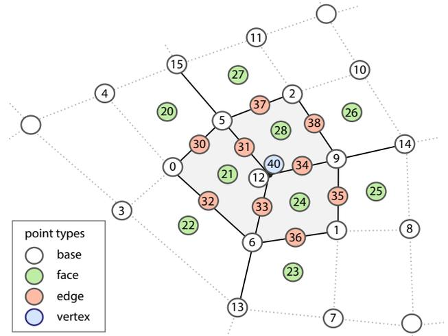
**Figure 4:** Simplified characteristic map for an irregular vertex with a valence of three. White points show the isolated base mesh for this characteristic map. Colored points refer to face points (red), edge points (green), and vertex points (blue), according to the Catmull Clark subdivision rules.
